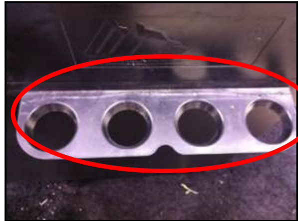
Metro Vision Plastic Tray with obvious attempt to glue the connector. (Greenbuild 2011)
